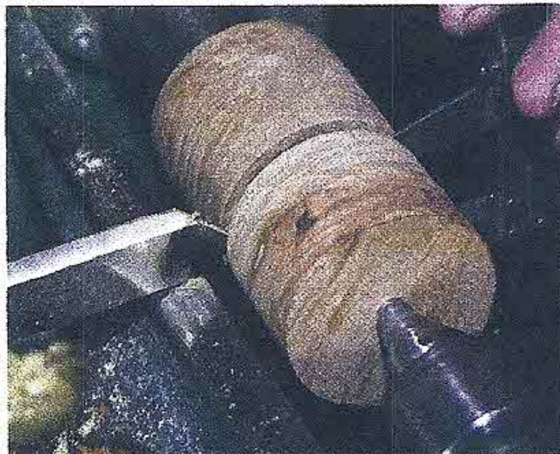
2 Making a 3mm ( \frac{1}{8} in) groove leaving a slightly smaller than 22mm ( \frac{7}{8} in) stub tenon to hold the globe onto the chuck fixing
