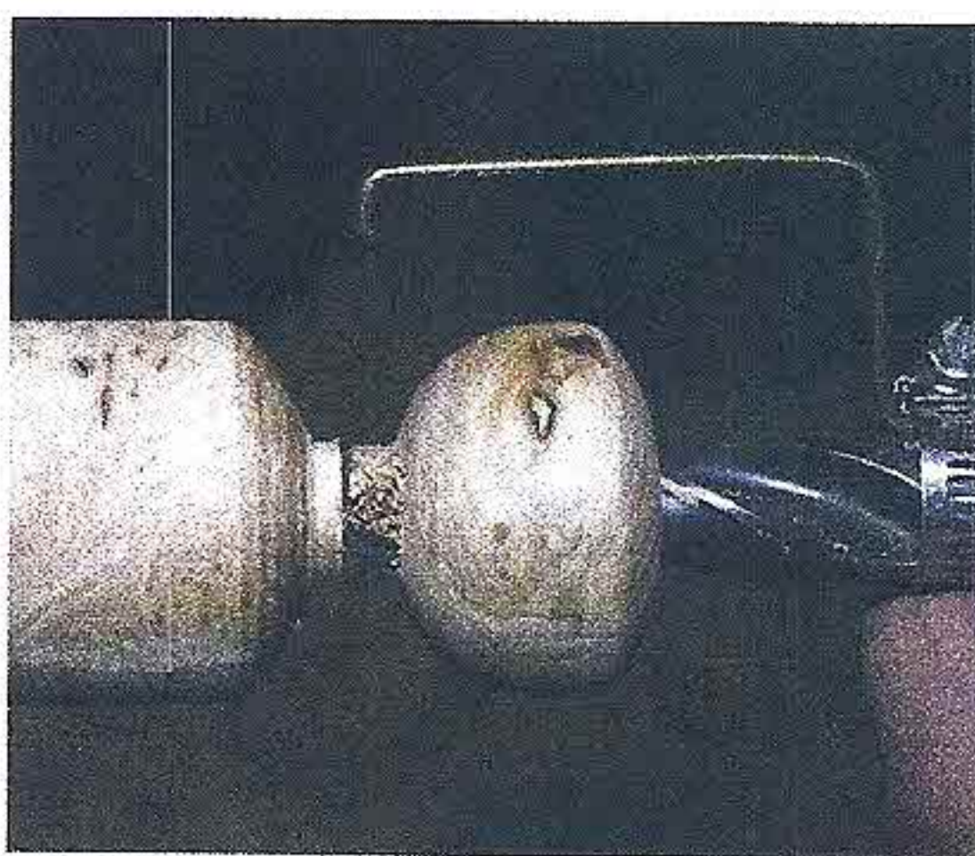
8 If the tenon holding the globe is turned to be a slightly smaller diameter than the 22mm ( \frac{7}{8} in) drill, the globe will neatly pop off on to the drill, removing the need to make a small parting cut
