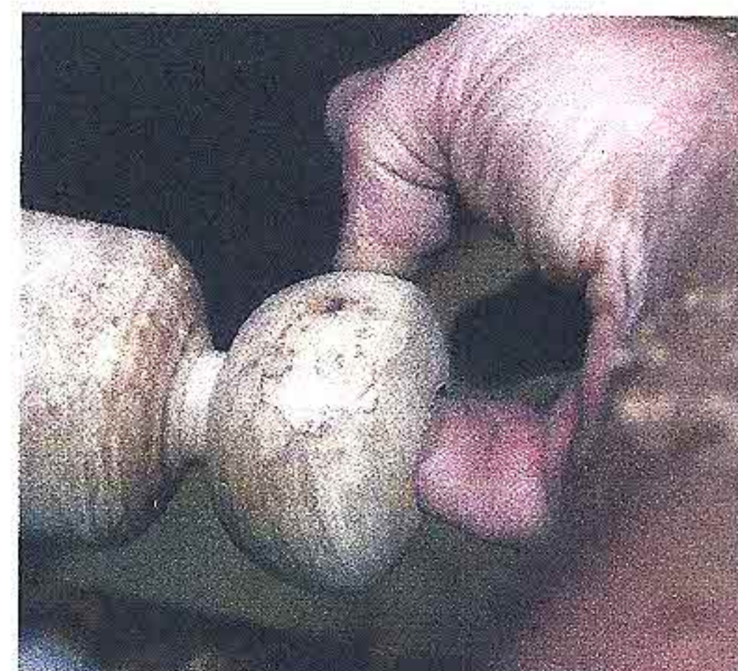
7 Using two fingers is a fast and surprisingly accurate way to caliper the wall thickness
